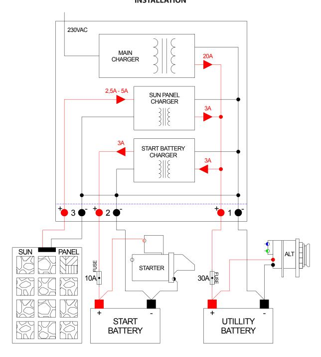
CCC12201203S03, Dual output 12V/20A and 12V/3A and input from sun panel:
