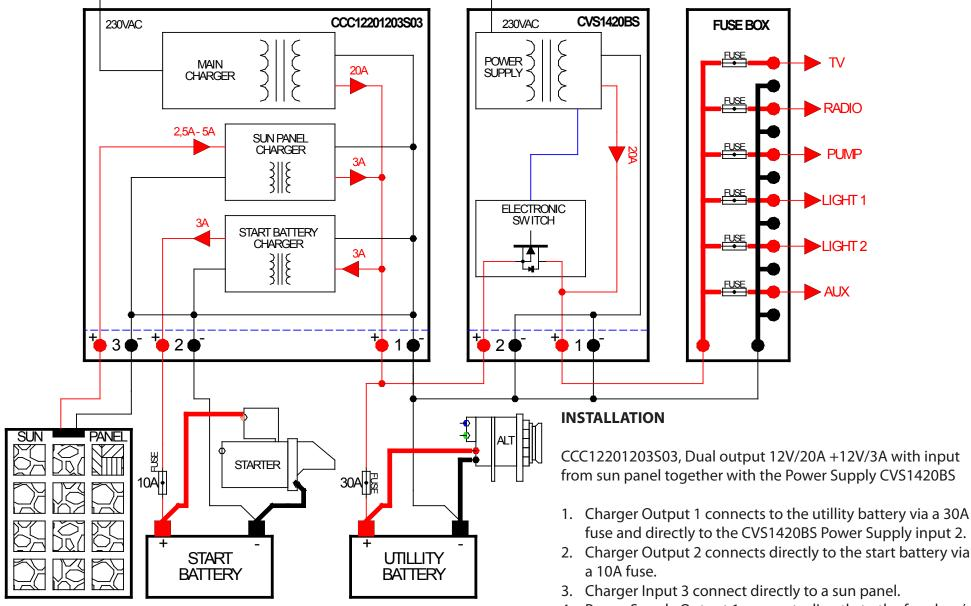
4. Power Supply Output 1 connects directly to the fuse box/ power distribution panel.
